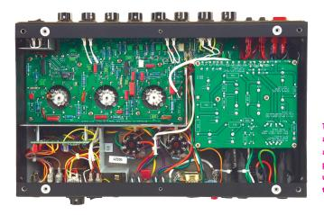
The Flexi-50 can accept a multitude of preamp and output tube types, providing an almost unlimited range of tone tweaking options.
